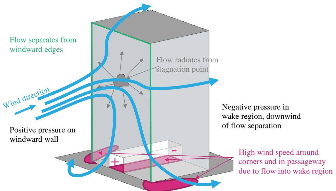
Figure 5 Schematic wind flow around tall isolated building
