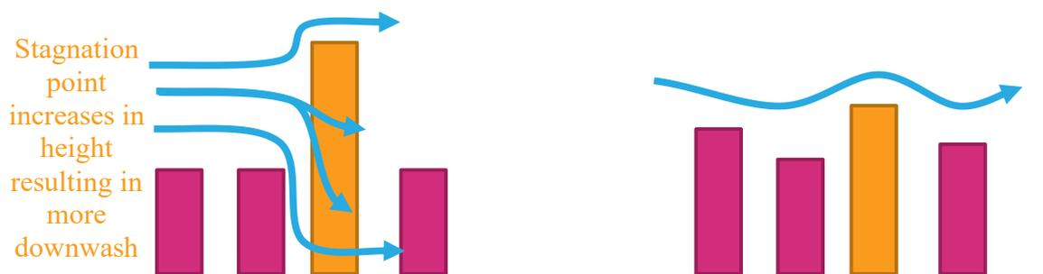
Figure 10 Schematic of flow pattern interference from surrounding buildings
