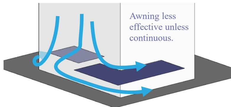
Figure 7 Schematic flow pattern around building with awning
